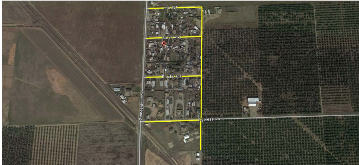
Figure 25. New pipeline for only potable water distribution to primary connections (yellow) and peripheral connections (blue) of Tonyville, CA (Google Earth © 2018 Google).
